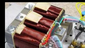
A standard three phase 400V alternator can supply 1/3 of its nominal power when used as single phase alternator. On EP6500T(E)-25 and on EP6500TLN generators, the alternator is wound with one reinforced phase, which enables the user to load the single phase socket up to 4kVA max.
