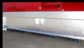
Especially in the rental business, the galvanised chassis is highly appreciated. The generating set keeps its original look and color, even when it has been loaded and unloaded hundreds of times.
