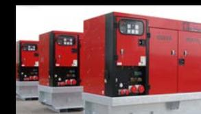
All Europower generators with electronic speed governor can run in parallel. The modules DSE 8610/8620/8660 are used for this purpose. 32 generators can run in parallel which allows rental companies to offer Megawatt power plants.
