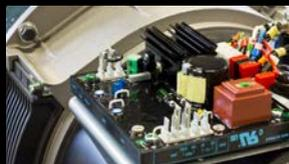
Optionally the generating set can be equipped with AVR. AVR stands for Automatic Voltage Regulator and maintains a constant and stable voltage.
