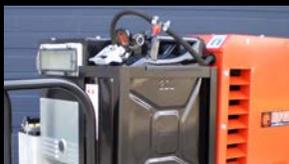
The two-cylinder generators with Honda engine are equipped with a 20 liter jerrycan that is easily interchangeable without stopping the engine.
