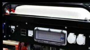
The control panel on all -25 types is easy to customize. The user can ask for integration of earth leakage protection or insulation protection. Voltmeter, hour counter and thermal magnetic protection are standard on these generating sets.
