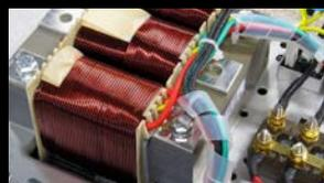
A standard three phase 400V alternator can supply 1/3 of its nominal power when used as single phase alternator. On EP5000T and EP6500T(E) generating sets, the alternator is wound with one reinforced phase, which enables the user to load the single phase socket up to 4kVA max.
