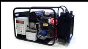
ECO A.I.S. stands for Automatic Idle System which means that the engine runs at idle speed when there is no load on the generating set. This technology leads to increased fuel efficiency and longer autonomy.
