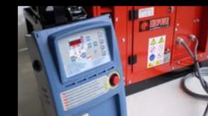
A.S.S.S. stands for Automatic Start/Stop System in case of mains failure: all generating sets with electric start can be equipped with this easy backup system, which has a built-in battery charger and computerized self-test.
